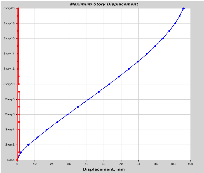
Figure.6: maximum displacement values of a building with X-bracing at outer and centre bays
