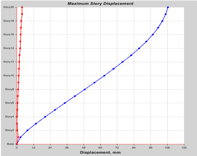
Figure.4: maximum displacement values of a building with V bracing at outer and centre bays
